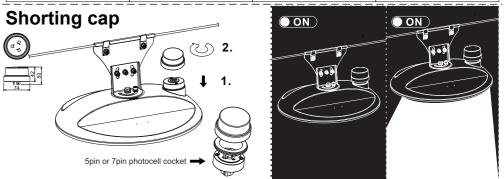
Note: If the luminaire use 5 pin or 7 pin photocell socket, it need to plus a waterproof
